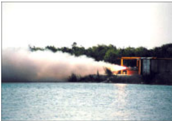
Figure 4b. Engine Firing Test (8000 lbf class)
